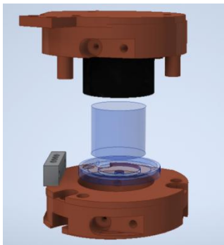
4 \pi veto, sensitive to holder transmitted events
