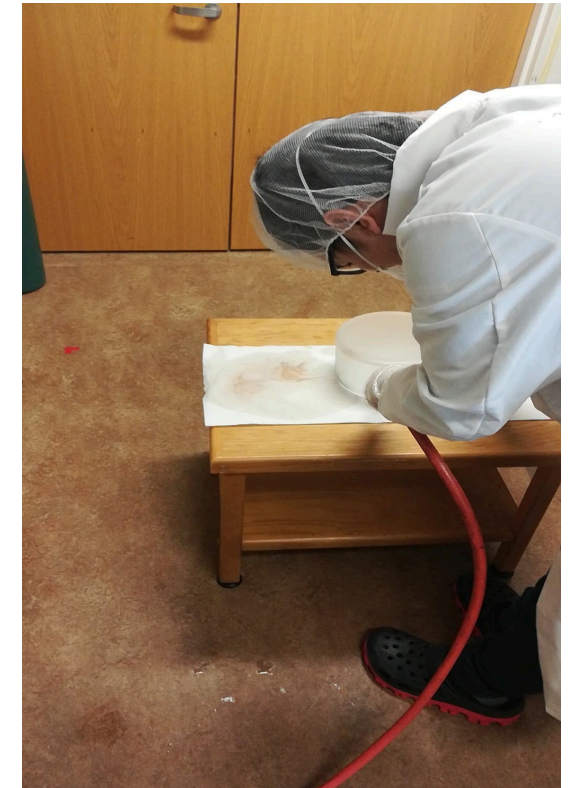
Drying with Nitrogen before loading in the chamber
