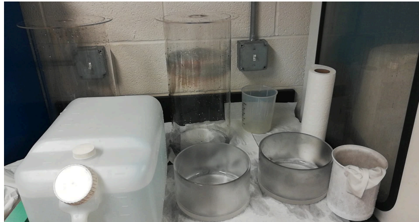
Crucible and glass tubes being cleaned with hydrogen peroxide
