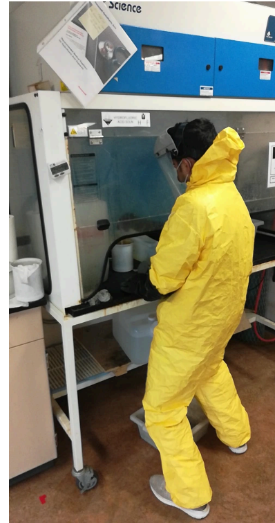
Etching ingots with strong acid, HF: HNO 3 (1:3)
