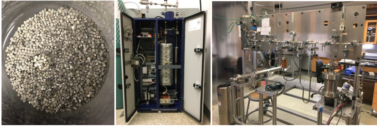
FIGURE 1. Left: St707 getter pills harvested from a used PS4-MT3 noble gas purifier. The darker pills in the lower right are oxidized from prior use. Center: The Entegris PS4-MT50 purifier. The getter pill vessel is inside the grey heater blanket on the right. Right: Radon transfer and counting system at the University of Maryland. Charcoal and copper traps are used to prepare clean helium and to collect and transfer the radon. The 1.7-liter ESC is the conflat vessel at lower right.
