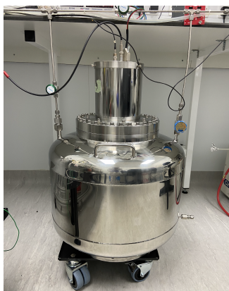
FIGURE 1. Image of the 80-L CREF electrostatic detector.
