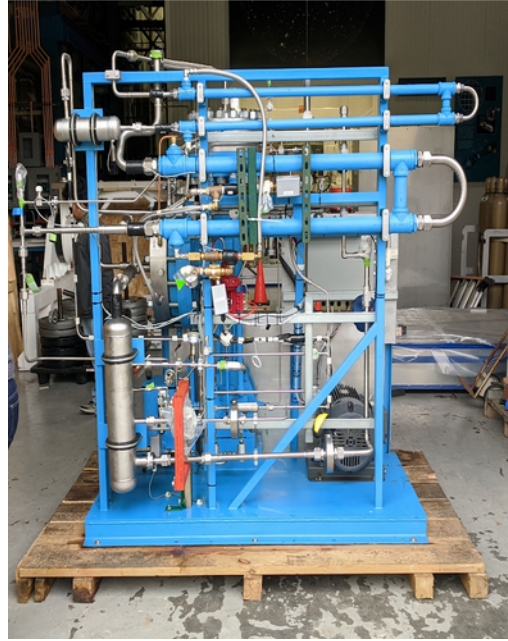
FIGURE 6: The Fluitron diaphragm compressor for xenon storage, shown prior to installation.
