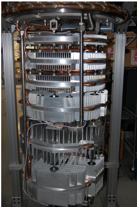
FIGURE 5: A photo of the freezer internals prior to installation, showing the finned aluminum plates for freezing xenon and the copper liquid nitrogen lines that provide cooling power.
