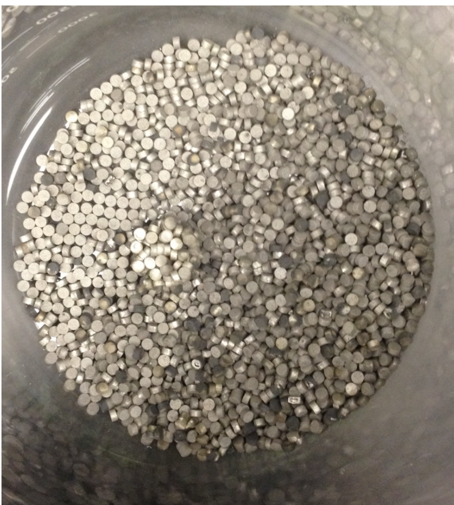
Left: St707 getter pills harvested from a SAES PS4-MT3 noble gas purifier. The shiny pills in the upper left are mostly unused; the darker pills in the lower right are oxidized from prior use. Right: SAES getter pill promotional brochure.
