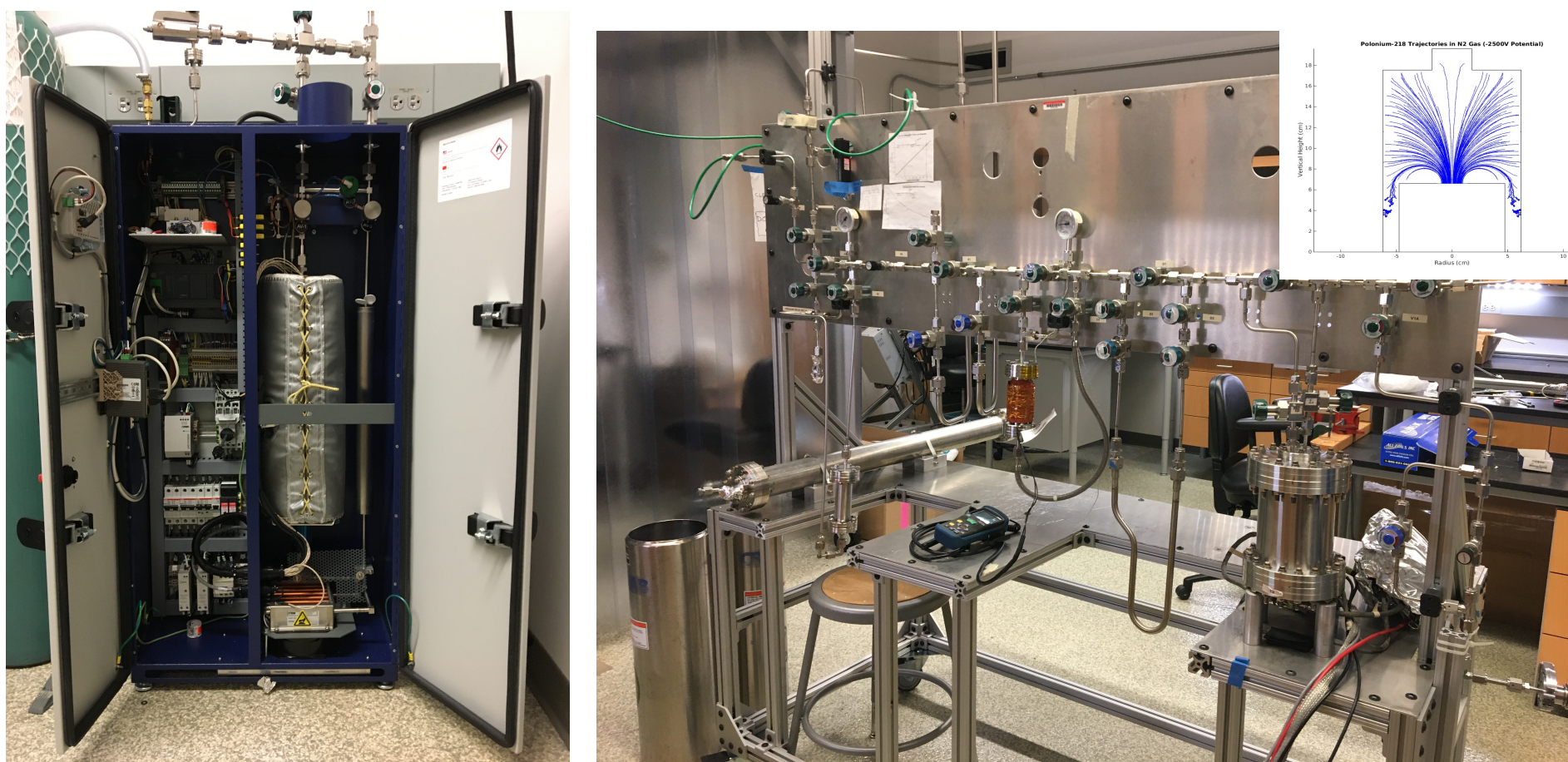
Left: The PS4-MT50 purifier at the University of Maryland. The getter vessel is inside the grey heater blanket on the right side. Right: Maryland Rn counting apparatus. Charcoal and copper traps are used to transfer Rn from the getter to the electrostatics counter (Conflat vessel at lower right). A silicon barrier detector (Ortec) is used to count 218 Po 214 Po, and other Rn daughters. Inset: A simulation of ion drift in the counter.
