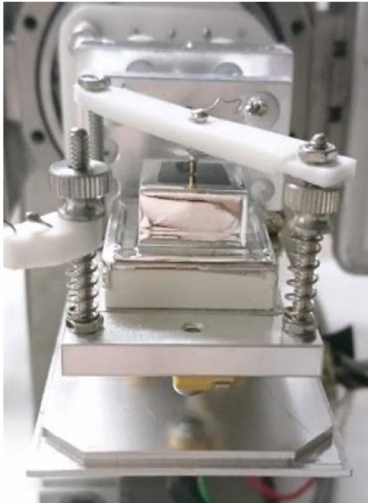
Shown is the detector USD-W06 loaded in a variable temperature cryostat for characterization.
