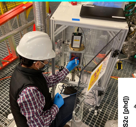
Mounting AmLi neutron source inside a calibration system
