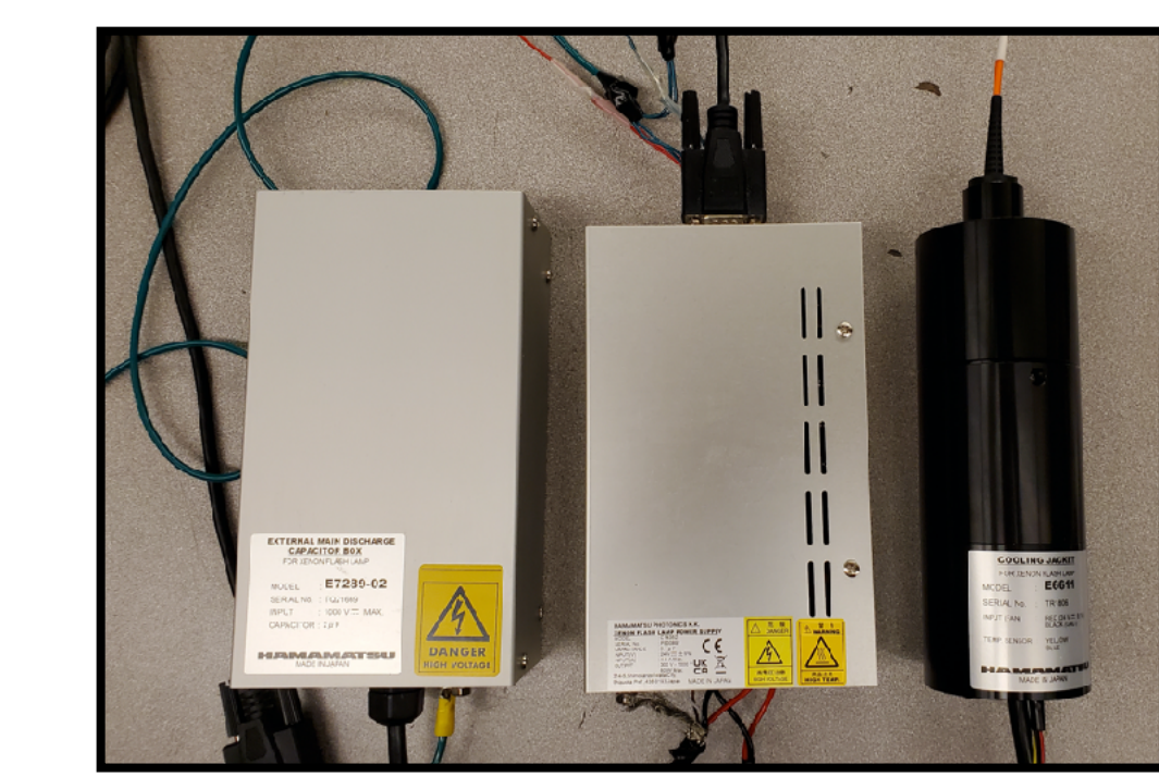
Fig. 5: 60W Xenon flash lamp being used to produce photoelectrons. Produces a flash of light within 10 \mu\text{s}
