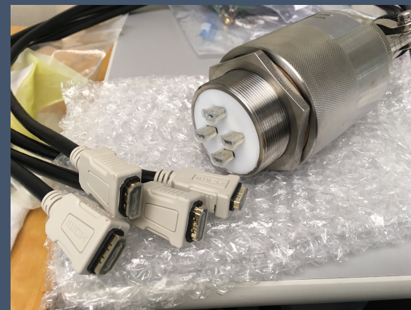
Digitize inside vessel, custom HDMI feedthroughs
