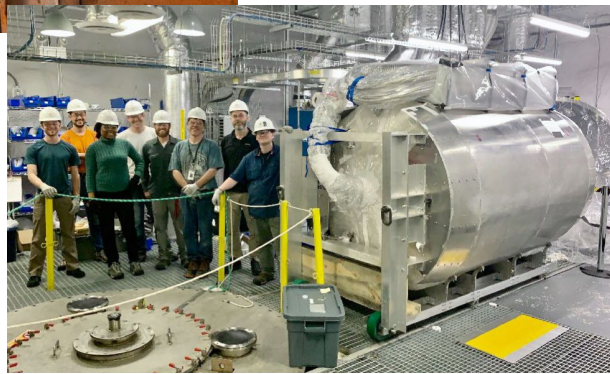
ICV, wrapped in insulation, entering the OCV
