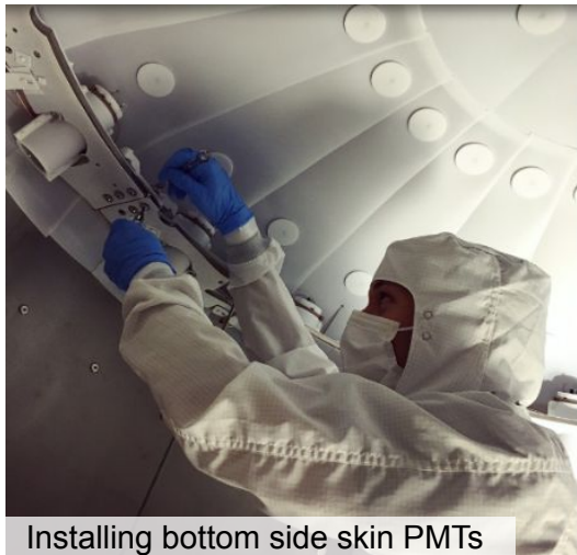
Inside of the ICV lined with PTFE
