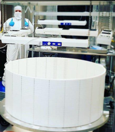
Field cage construction: the forward field region (FFR)
