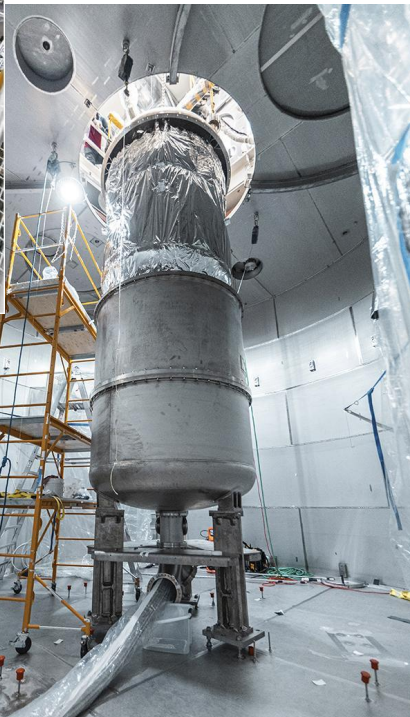
Connecting the cathode HV feedthrough and routing the cable bellows
