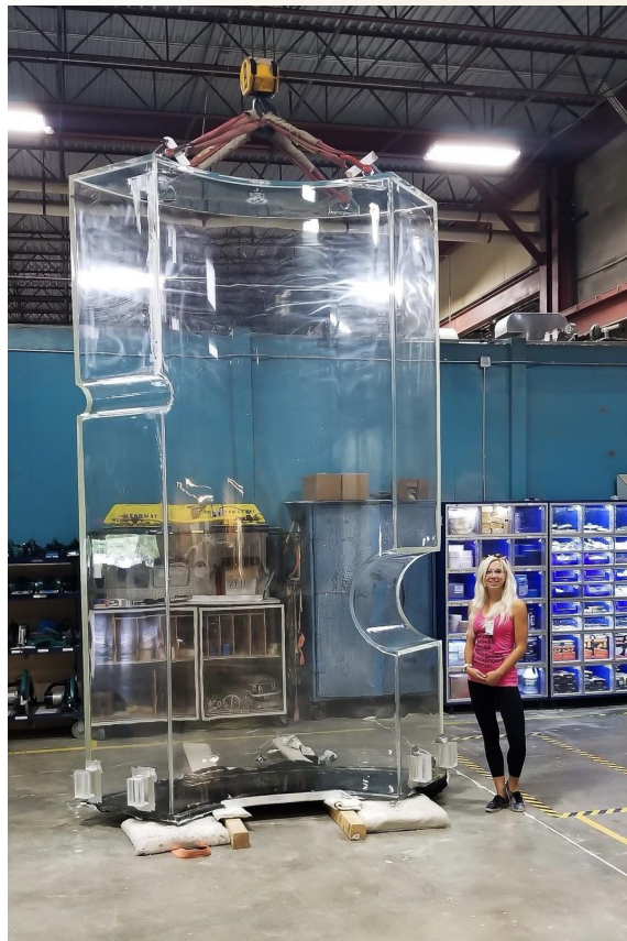
OD acrylic vessels surrounding the ICV inside of the water tank
