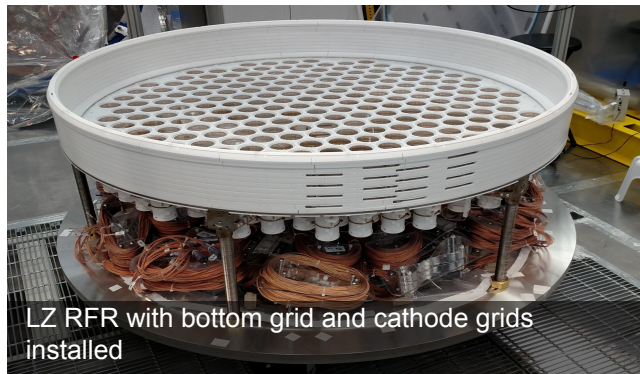
Bottom shield grid on top of the bottom PMT array
